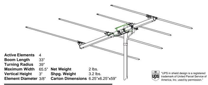
Output Impedance: 300 ohm / 75 ohm with included transformer Recommended Preamp: AP Series Made in U.S.A.
